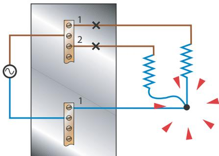
Lighting and control circuits are the most common examples where this practice is found. In these circumstances, the neutral conductor can become live when the conductor is disconnected, if a load is connected to that circuit.
